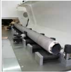
AUTOMATIC CUT-OFF OF SPUN IRON PIPES
